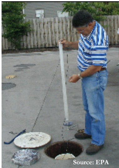
Ground water monitoring of UST secondary containment
