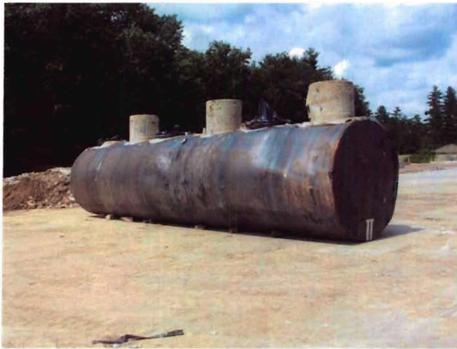
Photo 5 – View of 13,500-gallon UST with fiberglass coating removed.
