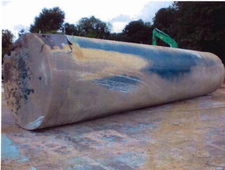
Photo 4 – View of bottom of 13,500-gallon UST.
