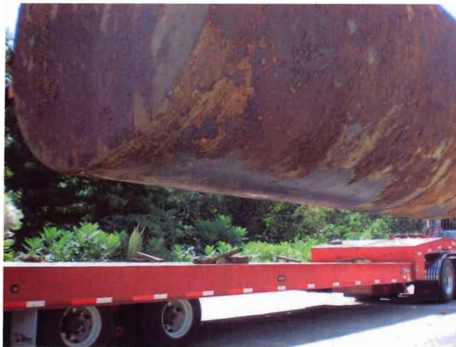
Photo 13 – View of bottom of 8,000-gallon UST.
