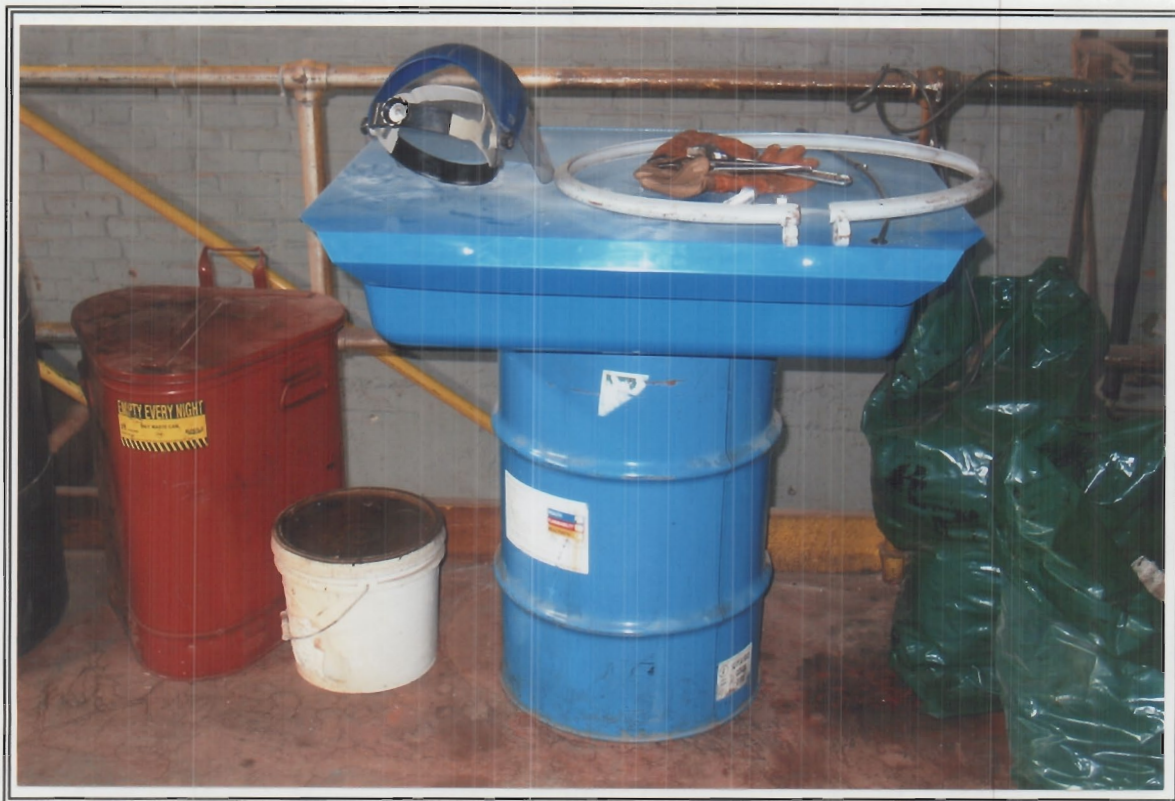
Photo 21. Parts washer (blue) and oily rag storage container (red) off of boiler room and near stairway to wastewater treatment room.
