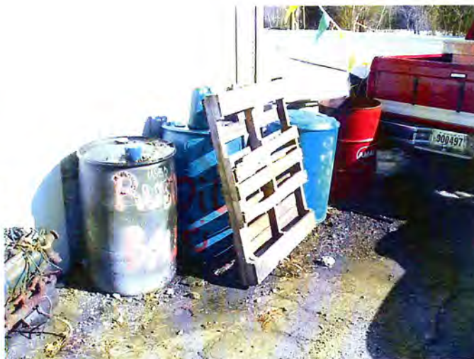
3 drums stored on top of stained soil
