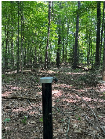
Photo 7: Monitoring Well in southwestern area of property
